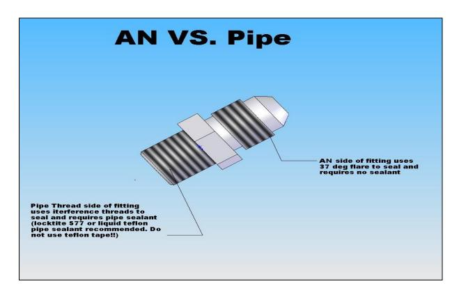
"AN" stands for Army Navy, which is a military spec type fitting. These fittings are sized by dash sizes, not fractional sizes.
